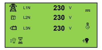
The module uses the same generator voltage inputs to sense the Mains supply voltages. The generator and mains switching must be controlled externally. When the *Mains Supply Active* digital input function is activated the module assumes the voltage sensed is the Mains supply. The *Mains Supply Active* signal must be connected through the mains switch auxiliary to feed the module's input, this ensures that when the mains breaker is closed the *Mains Supply Active* input is active.
